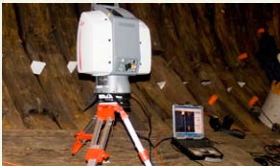
Above: 3D laser model of the ship Left: The laser scanner at work, linked to a laptop Right: The green laser beam scanning the timbers
